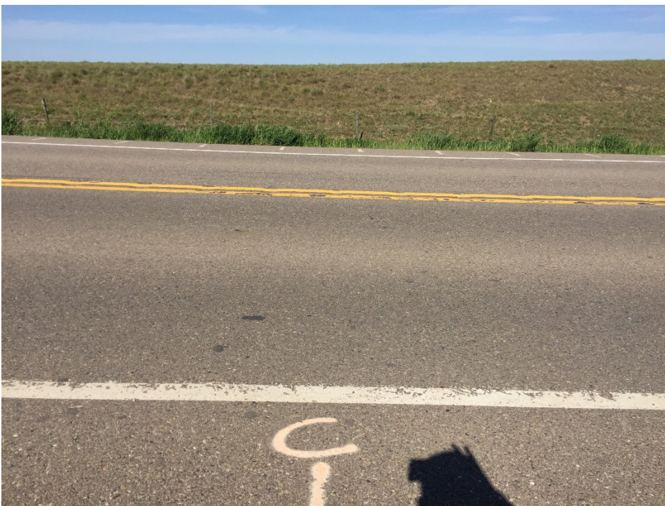
Photo 2 Survey pins installed in the highway in a grid pattern. Centerline of dip area marked on pavement. Photo was taken facing west on May 31, 2017.
