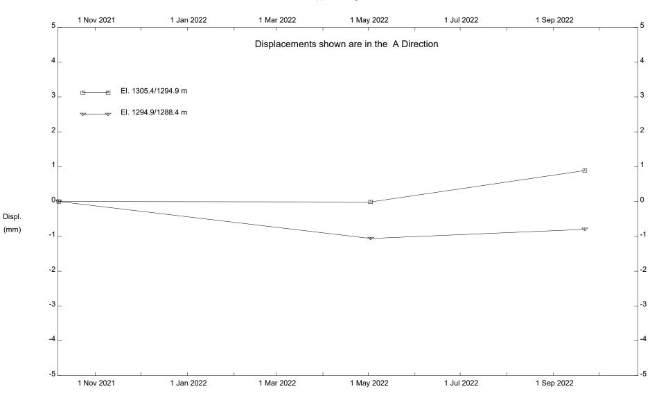
S008; H762:02, Fisher Creek, Inclinometer PILE36
