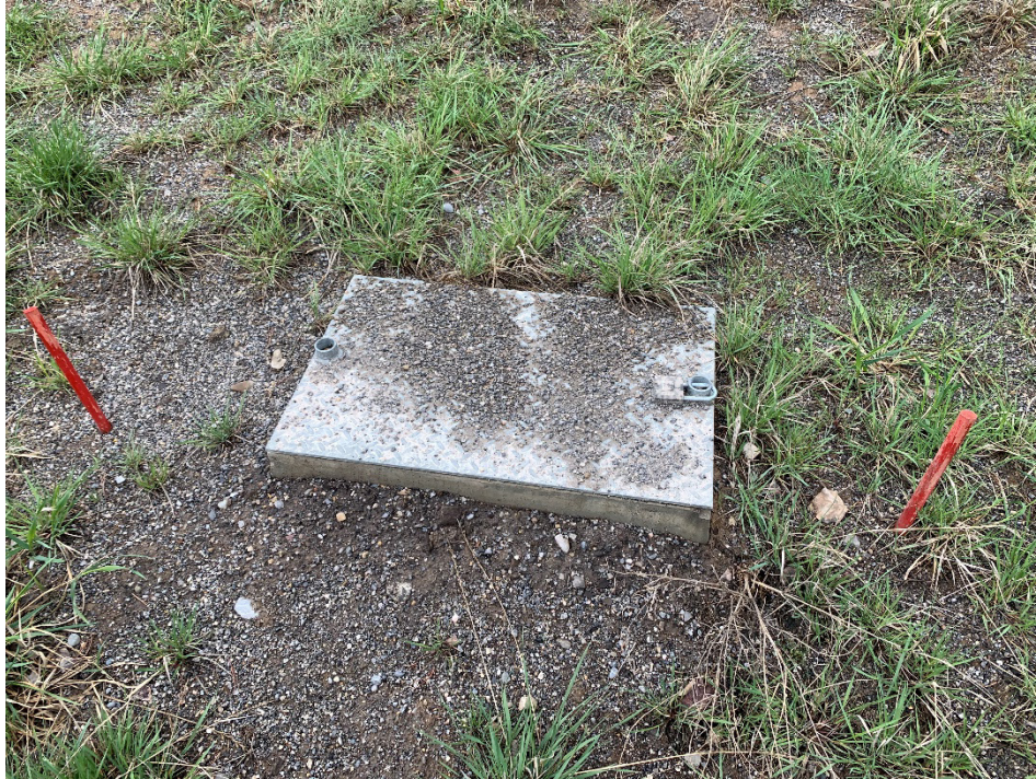
Photo 3 Headbox for Data Logger. Photo taken on north side of highway on May 8, 2023.
