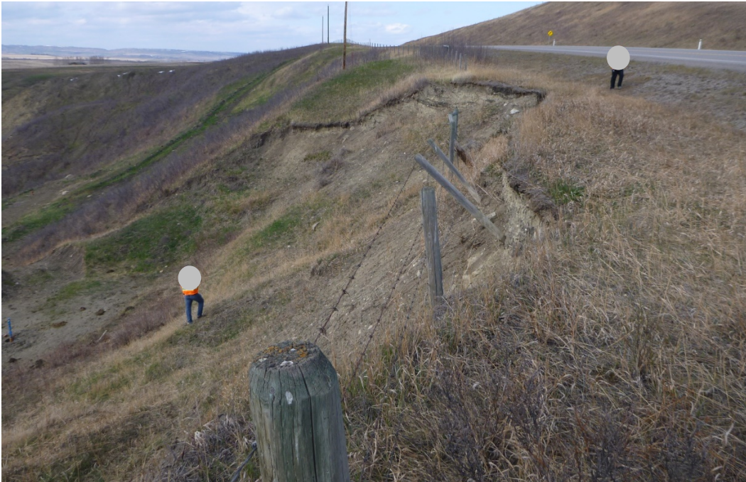
Photo 2 Site A: Instrumentation bench at mid slope of slide. Area around SI is wet. Photo was taken facing west on May 6, 2019.
