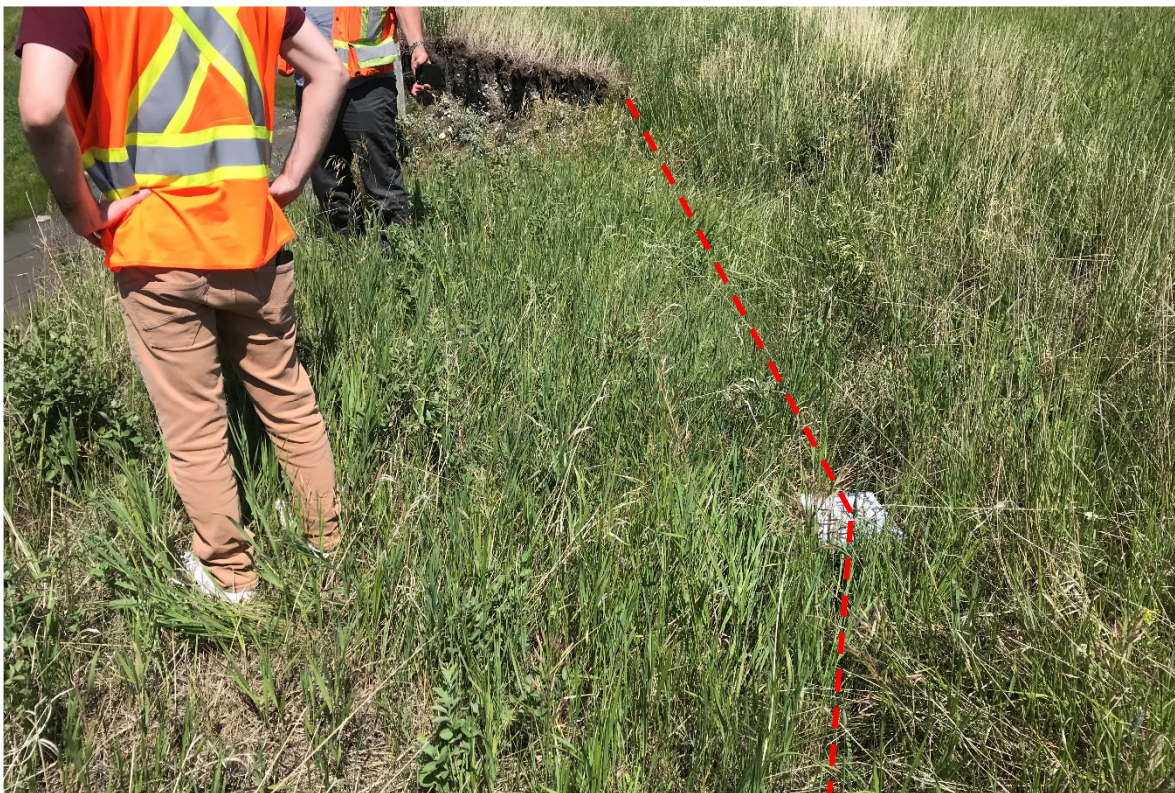
Photo 4 Tension cracking (red line) in highway right-of-way on the west flank of the erosion feature. Photo was taken facing northeast on July 9, 2021.
