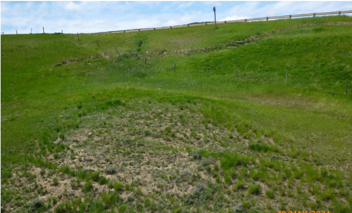
Photo 3 Head scarp on right flank. Photo taken on May 29, 2024, facing northwest.
