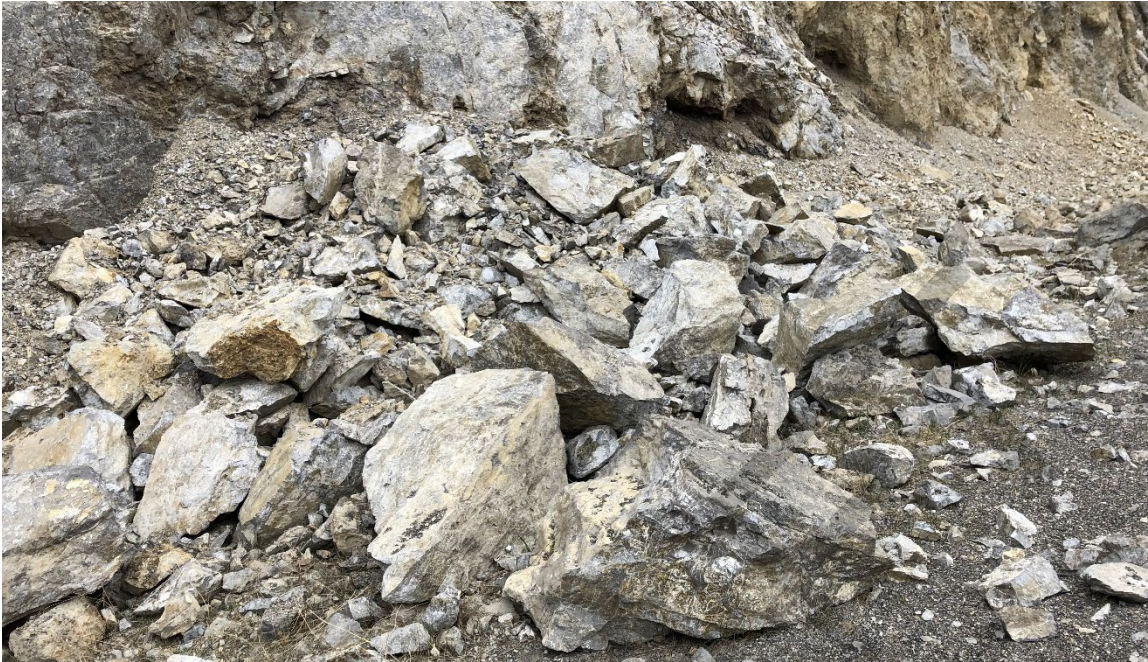
Photo 4 At the south end of the east rockfall site there is more severe weathering along the bedding planes leading to more overhangs that could lead to more rockfall debris. Photo taken May 17, 2022, facing southwest.
