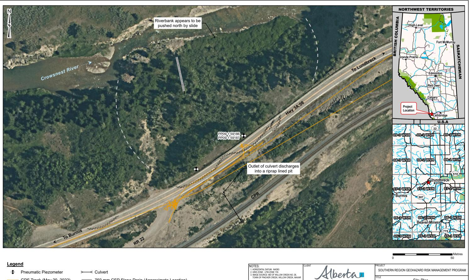
GPS Track (May 20, 2022) 750 mm CSP Slope Drain (Approximate Location)
