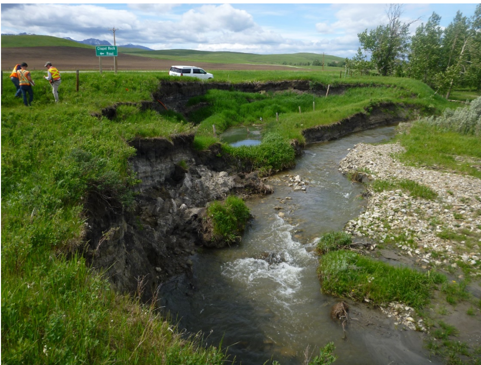
Photo 4 Site B - erosion scarp undermining fence with retrogressing back scarp instability approaching ditch. Photo was taken facing north west on June 1, 2017.
