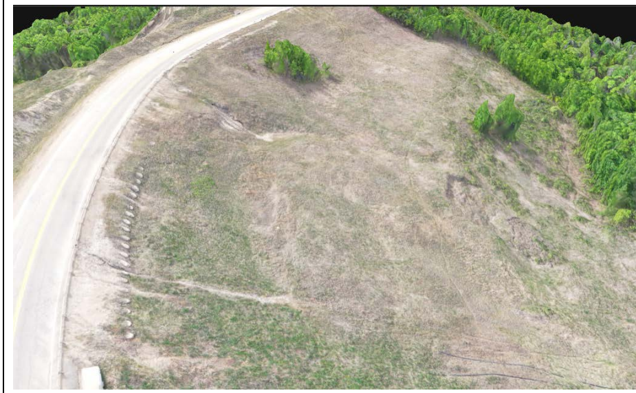
Photo 9. Screen capture from the 2023 drone photogrammetry model looking south towards the west slope below the highway near km 57.85. Recent slide activity is most apparent within the earth flows in the lower slope.
