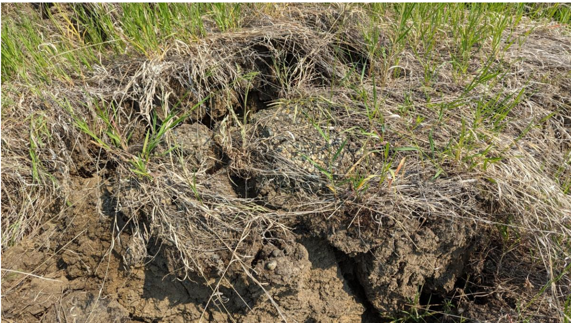
Photo 15B: Asphalt that appears to have been dumped or placed at ground surface and subsequently transported down the gully by the slide.
