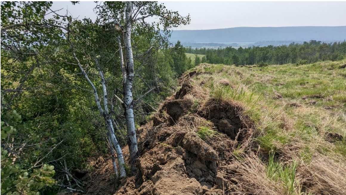
Photo 14: Looking south at eastern ridge of debris where it pushed over onto existing vegetation. The ridge is up to about 2 m high.
