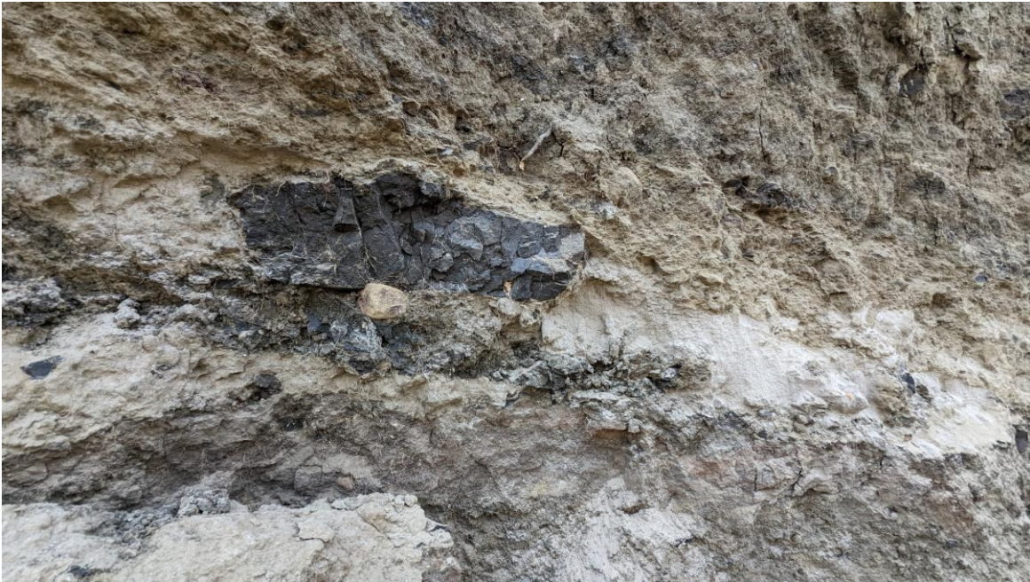
Photo 7: Pockets of fine sand and clay shale in the fill located on the east flank of the main headscarp.
