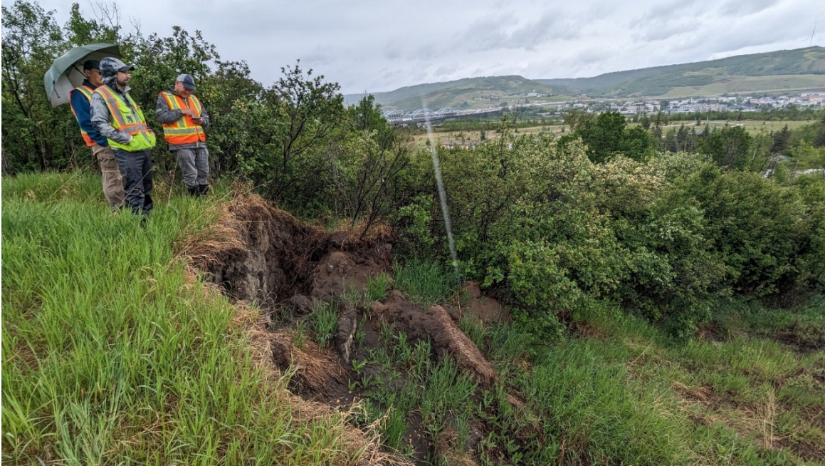
Photo 13: Looking north at the recent movement on the northwest flank of the active scarp. The CN rail line is located downslope of this landslide.
