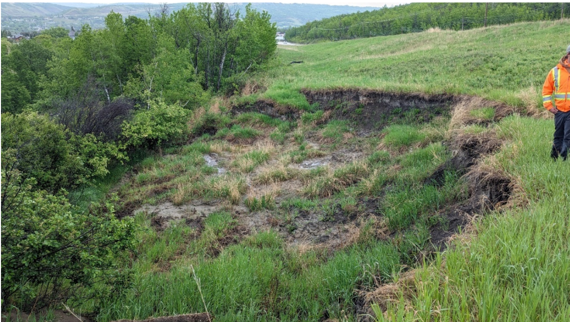
Photo 12: Looking southeast at the active scarp just beyond the edge of the highway ROW.
