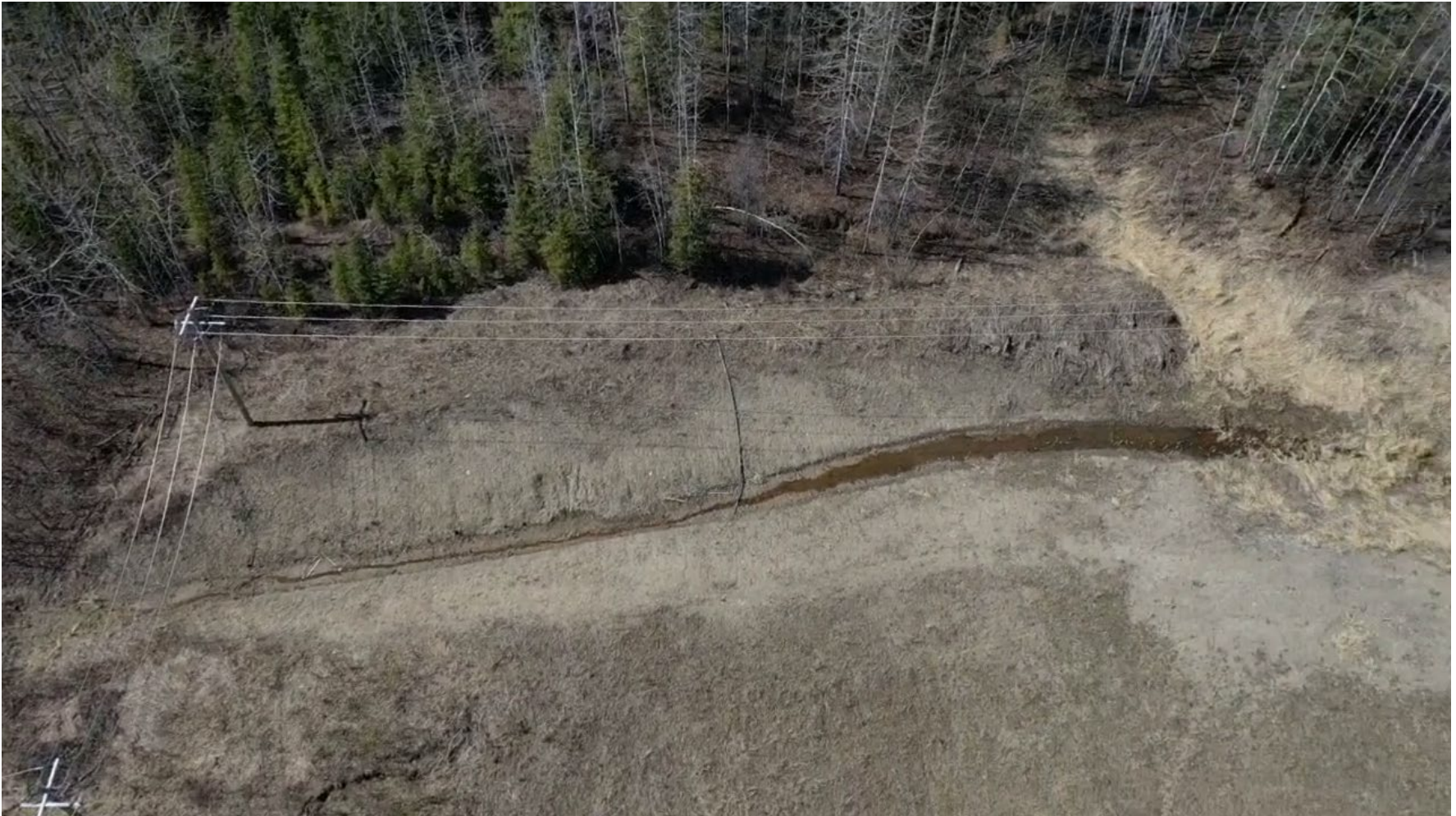
Photo 5 Diversion ditch on crest of backslope. Photo taken with UAV on May 9, 2024, facing west near south end of the GP044 site.
