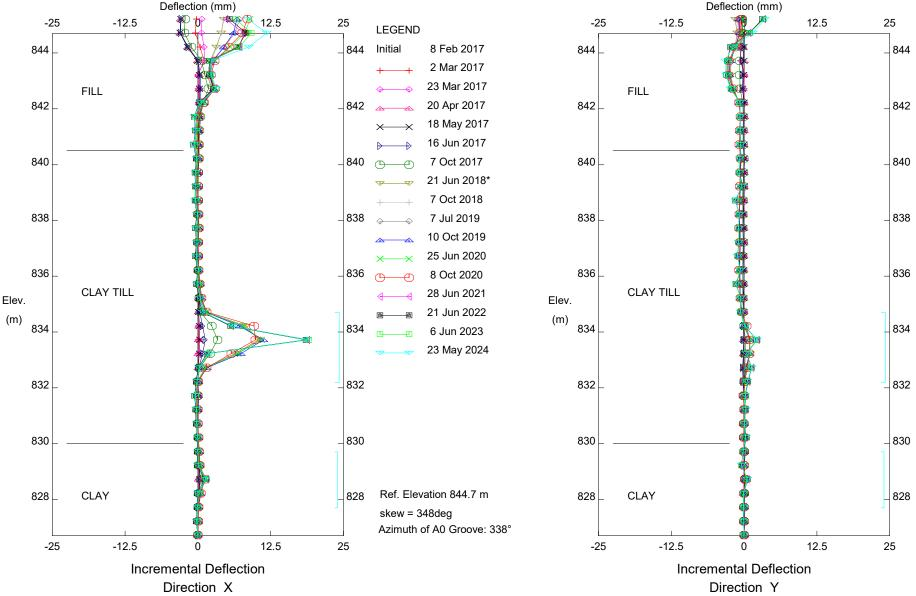
GP038-I; H40:38, Kakwa River Bridge, Inclinometer SI17-1
