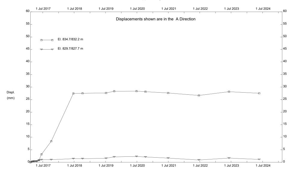
GP038-I; H40:38, Kakwa River Bridge, Inclinometer SI17-1
