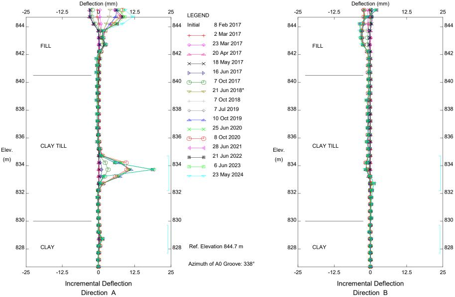
GP038-I; H40:38, Kakwa River Bridge, Inclinometer SI17-1
