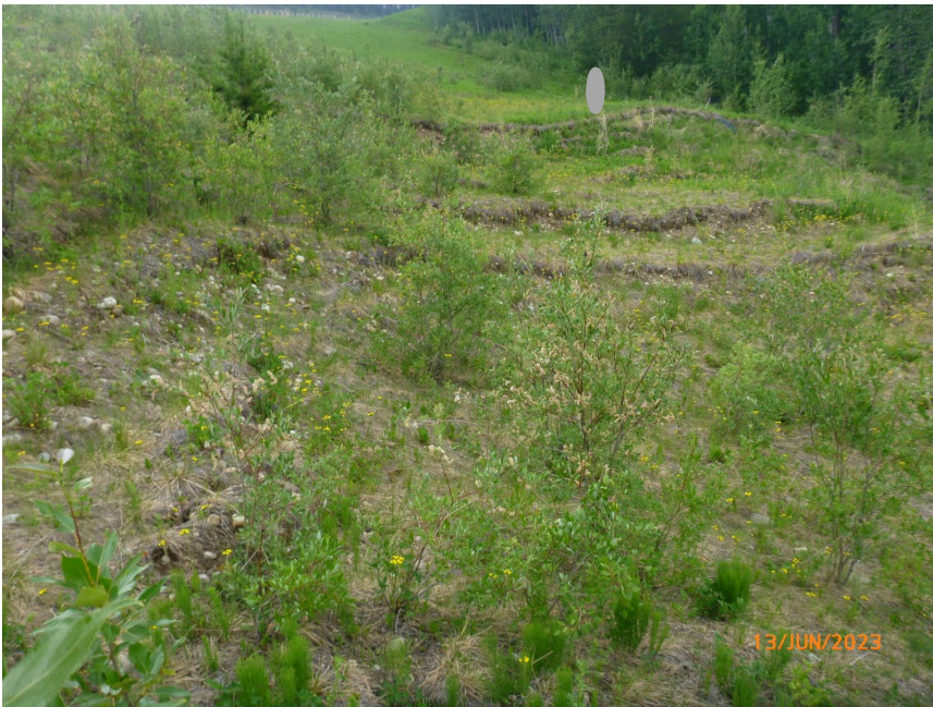
Photo 4 Looking across middle of slide from south/right flank near WP303. Note subrounded to rounded gravel and cobbles exposed on slope. Photo taken June 13, 2023, facing north.
