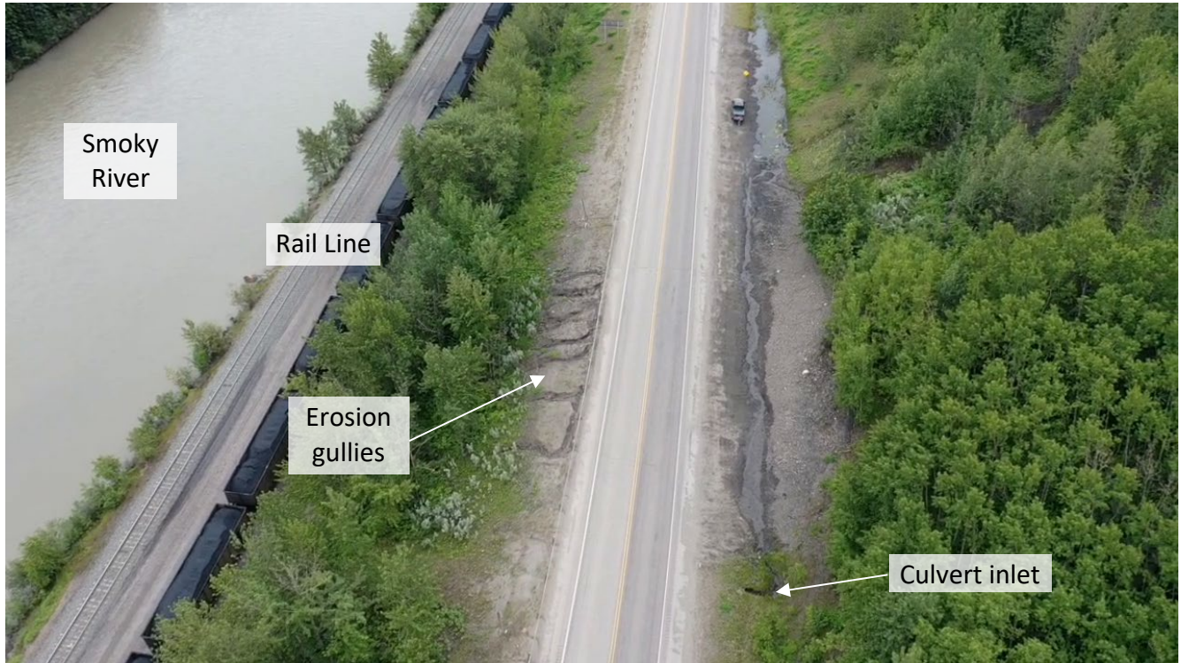
Photo 2 Overview of debris flow site. Photo taken with UAV on June 26, 2024, facing southwest.
