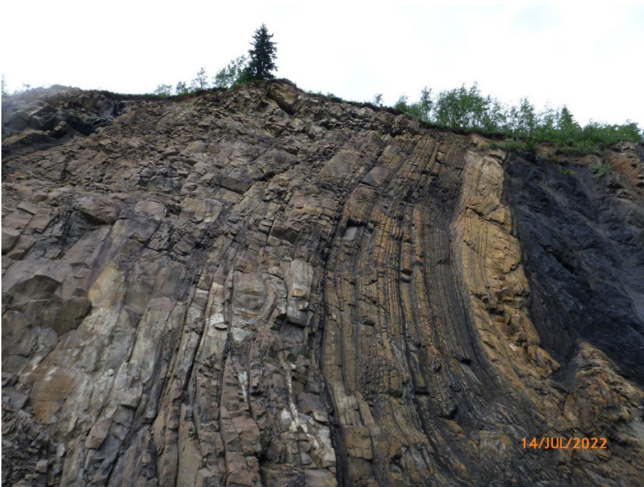
Photo GP036 – 12 More competent section of rock slope between coal seams (adit coal seam is to the right (north)). Photo taken July 14, 2022, facing northwest.
