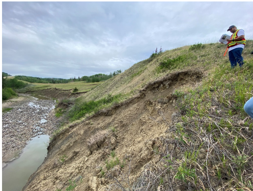
Photo 3. Looking west at area that sloughed into the creek. Photo credit: Don Proudfoot.
