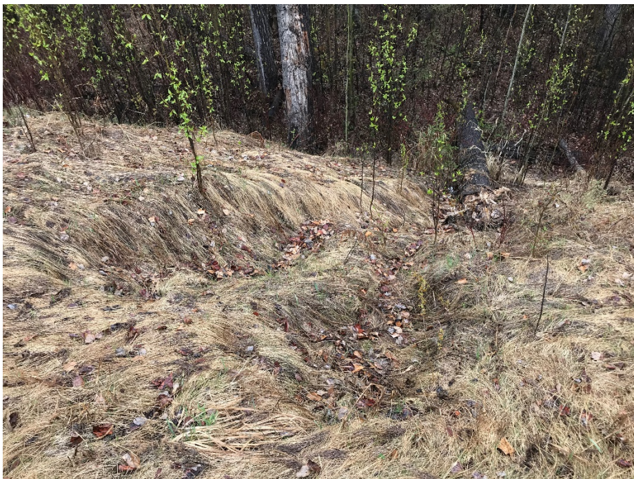
Photo 16: One of a series of about 10 slump/erosion features about 150 m west of Photo 12 at toe of slope. Looking north.
