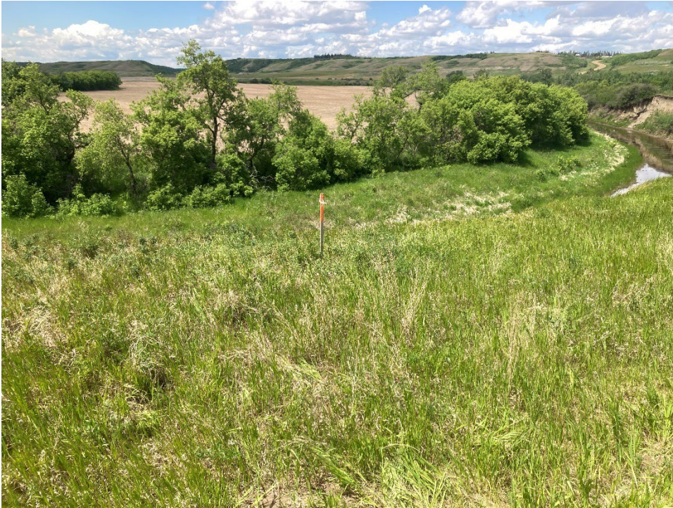
Photo 8 Stake 3 (southmost stake, location indicated by red circle) installed approximately 1.7 m from the near-vertical erosion face to monitor rate of erosion. Photo taken June 17, 2024, facing southwest.
