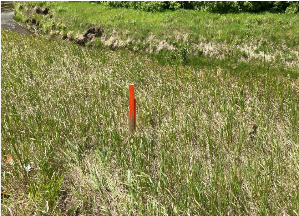
Photo 6 Stake 1 (northmost stake) installed approximately 1.6 m from the near-vertical erosion face to monitor rate of erosion. Photo taken June 17, 2024, facing west.
