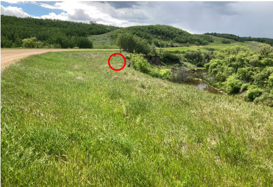
Photo 8 Stake 3 (southmost stake, location indicated by red circle) installed approximately 1.7 m from the near-vertical erosion face to monitor rate of erosion. Photo taken June 17, 2024, facing southwest.
