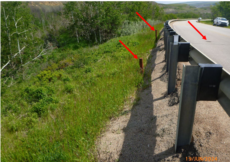
Photo 13 The three slope inclinometers (2017 and 2021) installed at the C065-4 site. Locations indicated by red arrows. Photo taken June 19, 2024, facing east.
