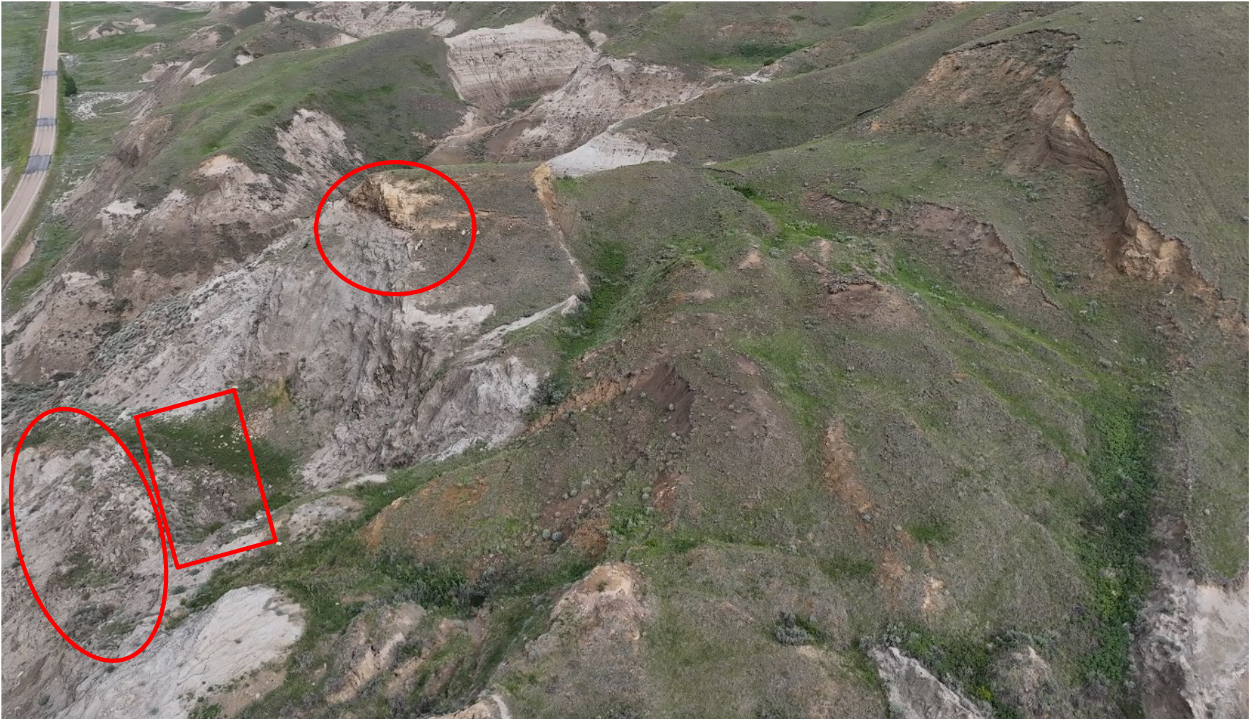
Photo 4 Aerial photo of the upper portion of the slope. Area where new ground cracks were observed indicated by red rectangle and areas previously scaled in 2022 are indicated by red circles. Photo taken June 18, 2024, facing west.
