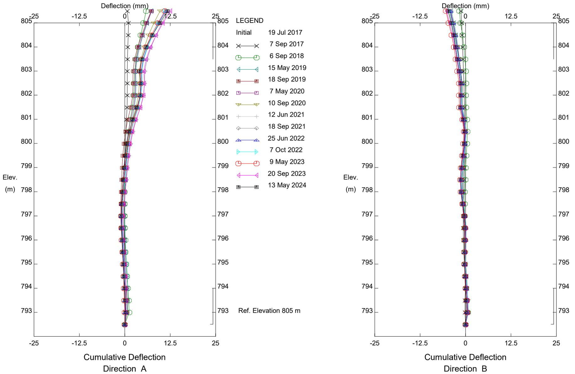
C067; H21:14, Kneehill Creek Slide, Inclinometer SI17-C67-05
