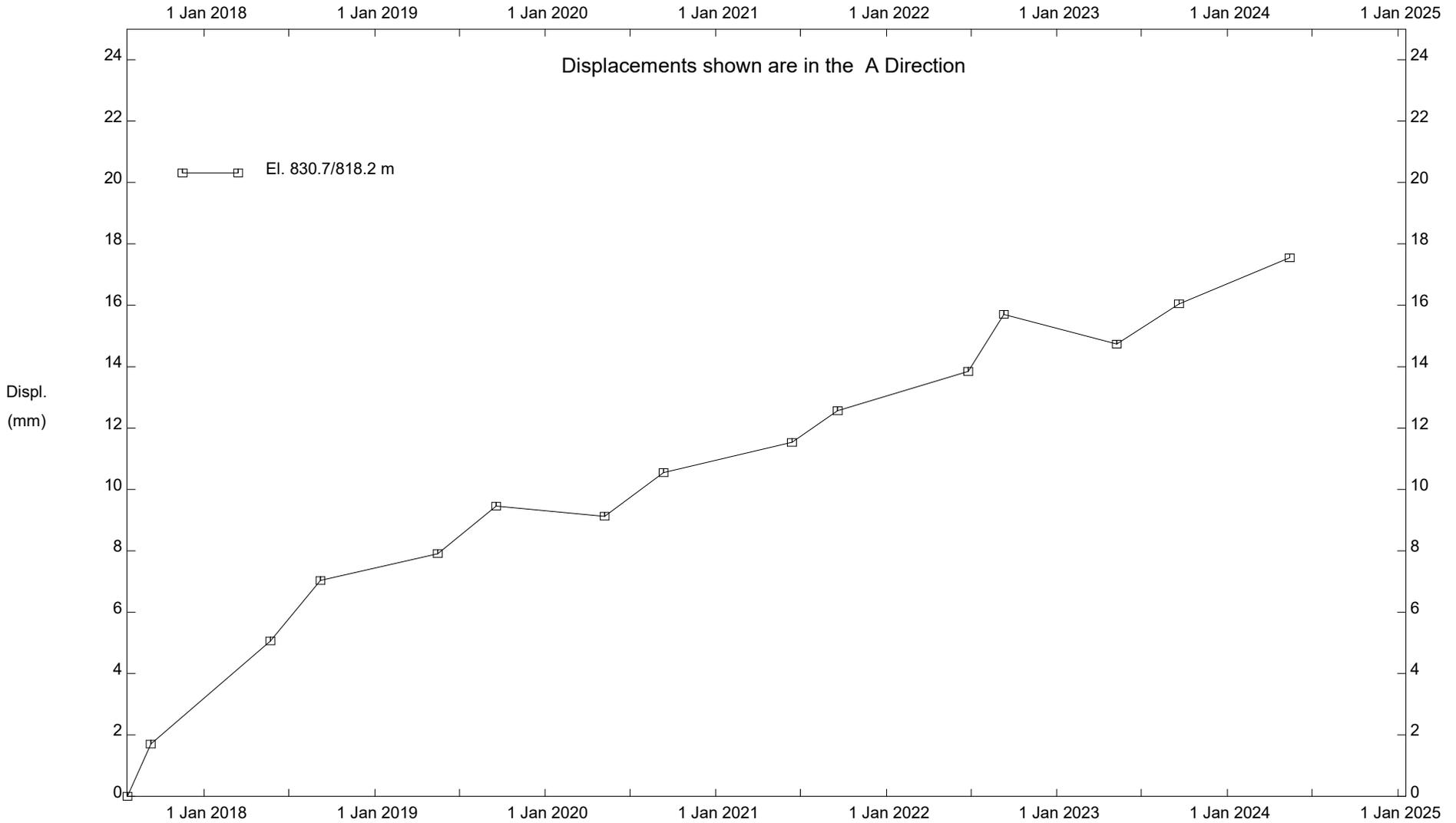
C067; H21:14, Kneehill Creek Slide, Inclinometer SI17-C67-02
