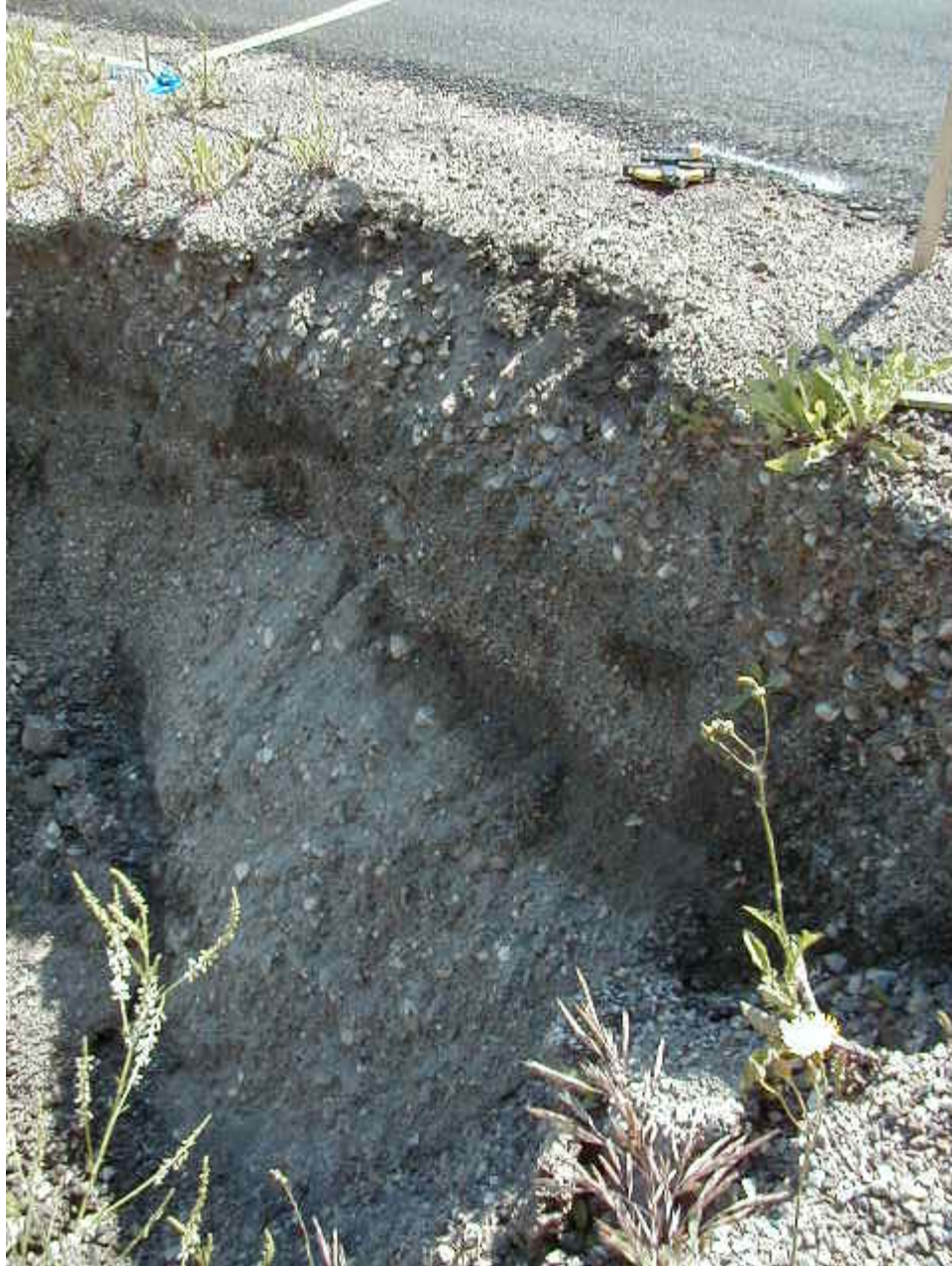
Main scarp of slide. Scarp is about 4 m wide and 2 m high. Note darker band at about mid-height which is a saturated sandy seam.
