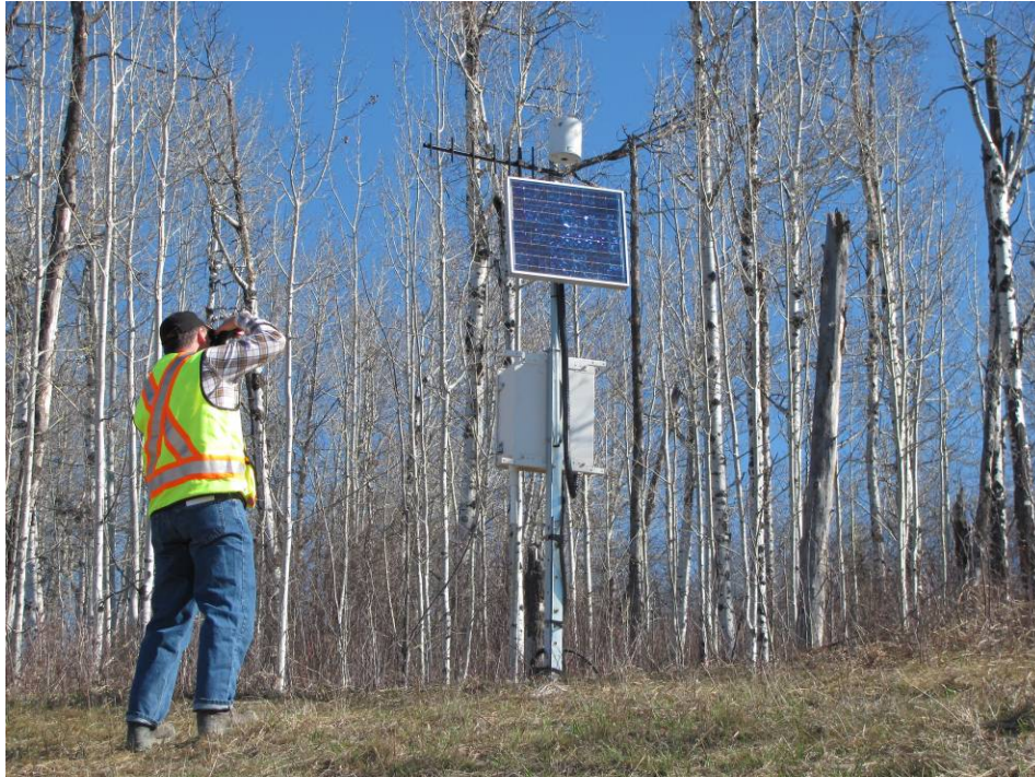
Photo #1 Looking at the weather station installed at NC 14
