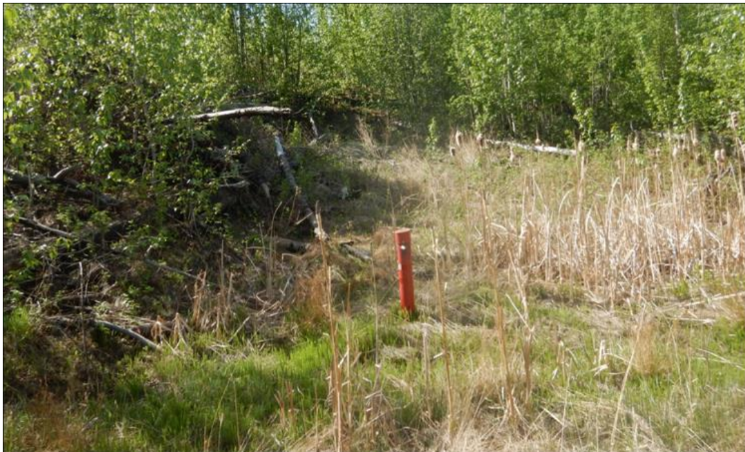
Photo 6. Looking northwest at backscarp; note cattails and lush vegetation due to seepage near SI17-3.
