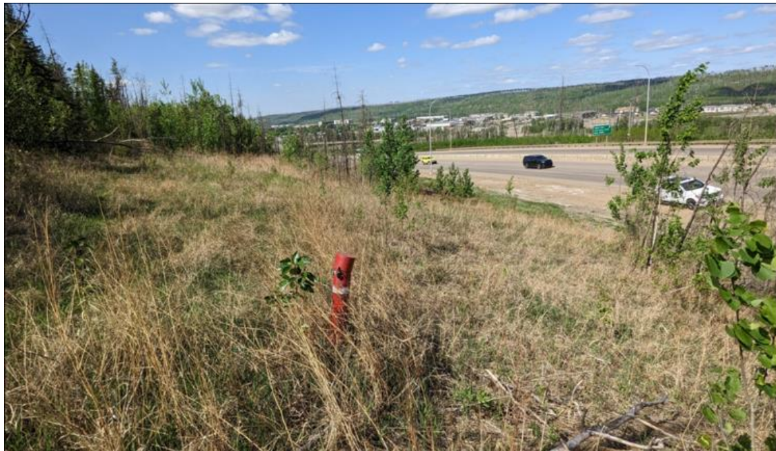
Photo 4. Looking south at the toe of the landslide; note tilting trees within the landslide mass.
