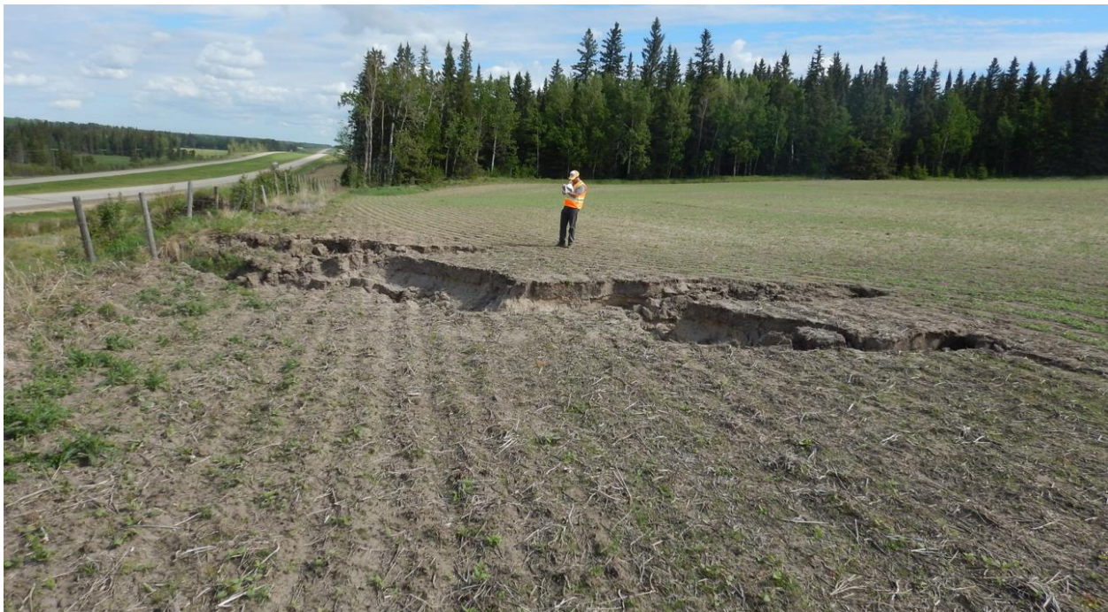
Photo No. 2- NC091-1: Looking north at a 12 m long erosion gully developed within the farmer's field; note the presence of sandy soils within the exposed surfaces of the gully walls
