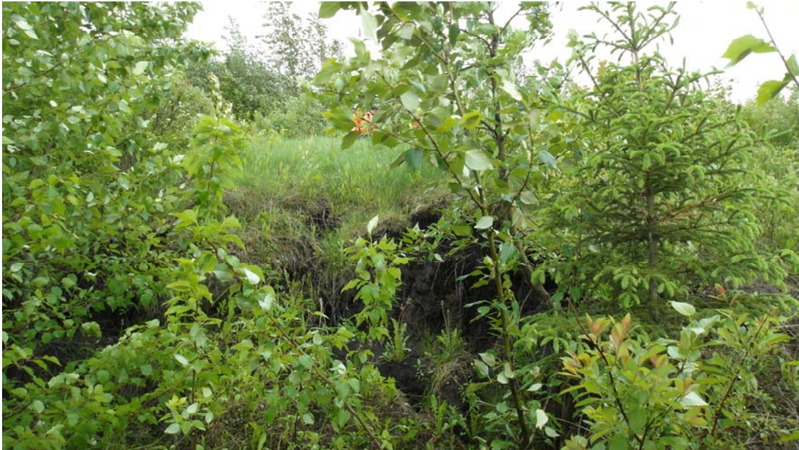
Photo# 3 Looking south at the north facing crack; note fresh scarp and slight retrogression of the slump
