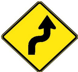
The Reverse Curve sign is used in advance of a roadway alignment consisting of two curves in opposite directions separated by a tangent section of 120 m or less. Each curve in the reverse curve segment must meet the requirements for a Curve sign, as defined in Table 1, included in the guideline for Turn and Curve Signs.
